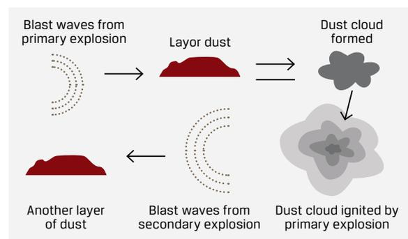
Where ignitable Carbon Black dust / air mixtures are handled, equipment has to be classified according to hazardous area classifications [13-16]. Ignition sources that exceed the MIE of Carbon Black have to be strictly avoided.
