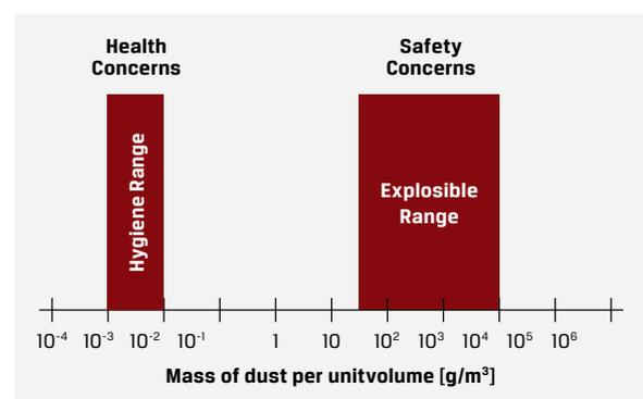
industrial hygiene limits which typically have threshold limits below 0.01 g/m<sup>3</sup> (e.g. United States, OSHA, PEL: 0.0035 g/m<sup>3</sup>). Dust concentrations greater than 50 g/m<sup>3</sup> usually occur only inside equipment, provided that handling is properly performed and industrial hygiene instructions are obeyed [8].
